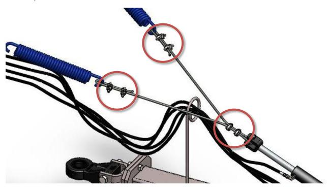
• With all personnel clear, run the hydraulics to be sure the puller is straight off the back of the tractor when raised. If you need to make any adjustments, lower the puller all the way to the ground to relieve all spring pressure before you loosen any clamps.
