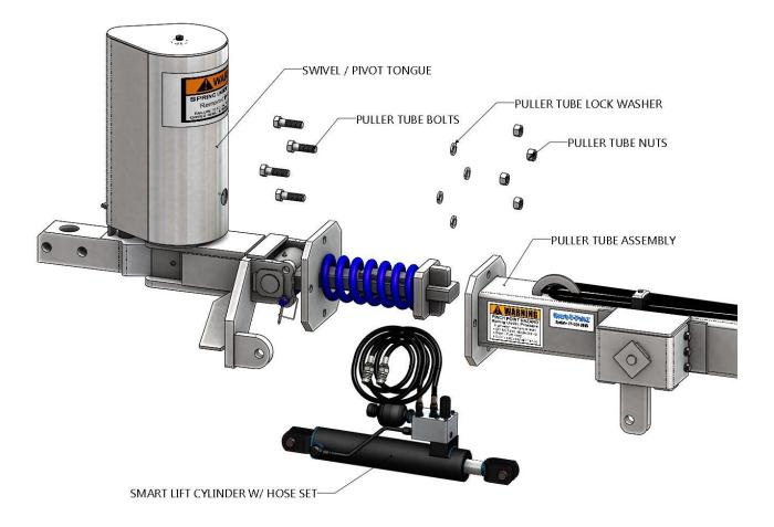
**Step 5**: Using the provided pins, attach the *Smart Lift Cylinder* as shown below.
