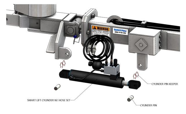
**Step 6:** Attach the hydraulic hoses to the *Smart Lift Cylinder*. Note: Two 11/16" wrenches required
