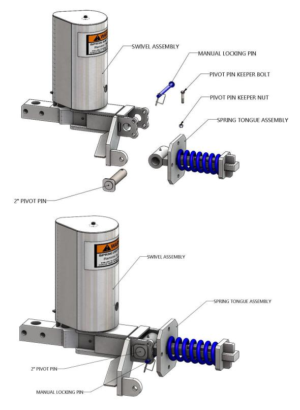
**Step 3:** Align the puller tube assembly and swivel assemblies as shown below. Slide the Spring Tongue into the Puller Tube Assembly.
