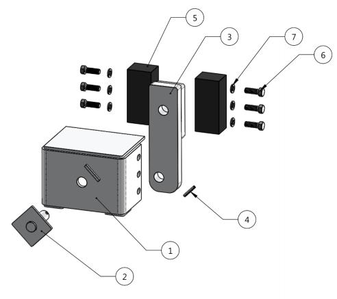
BOM #5 SAFE-T-PULL TORSION BOX REPLACEMENT PARTS
