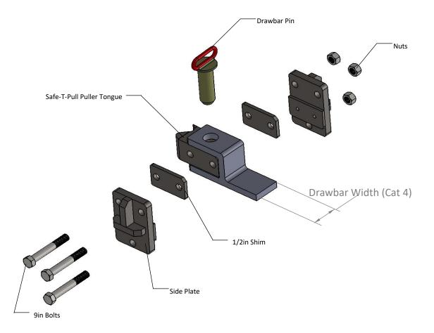
**Step 2:** Slide your tractor's pin into the drawbar. Be sure to use the correct bushings according to your drawbar width and pin size.
