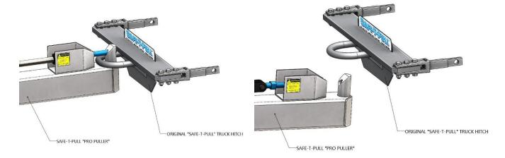
To unhook, open the latch pin, lower the puller arm, and drive away.
