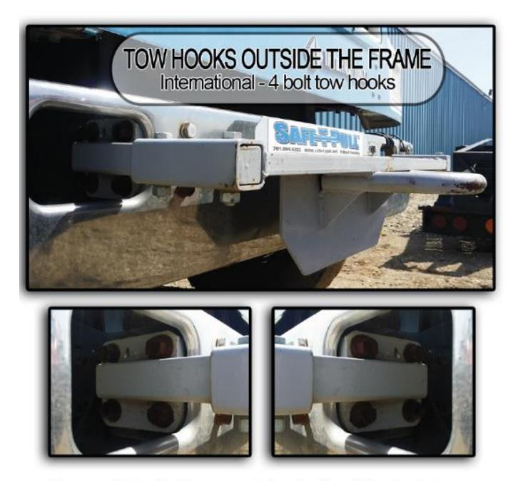
Measure outstide of the frame across to the other frame. These tow hooks are typically a 4 bolt hook with a square pattern.
