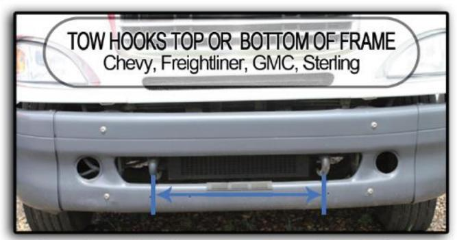
Measure tow hook bolts from one frame rail across to the other tow hook
