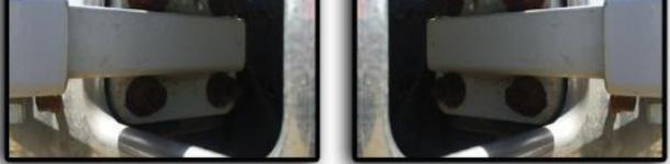
Measure inside of the frame across to the other frame. These tow hooks are typically a 4 bolt hook in square or rectangle pattern.
