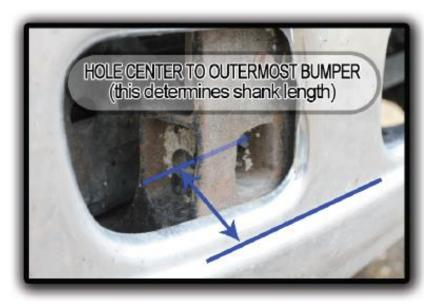
Freightliner Typical bar widths - 32-1/4", 44-1/4", 46-1/4", 49-1/2" Typical shank length - above measurements have one standard length
