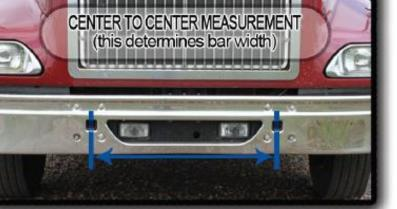
Step 1: Measure center to center across the square receivers to determine the frame width & bar length needed.
